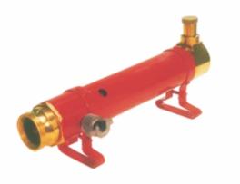
Inline foam generator is modified version of Inline inductor. It inducts foam as well as expands it and also transports the foam a long distance
